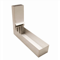
SCC - L Shape Box Apparatus
