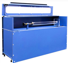
Sand Equivalent Shaker
